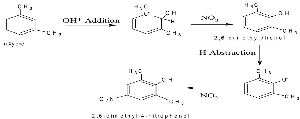
**Figure 2.4:** Formation mechanism of 2,6-dimethyl-4-nitrophenol from xylene (Zhao et al., 2005)
