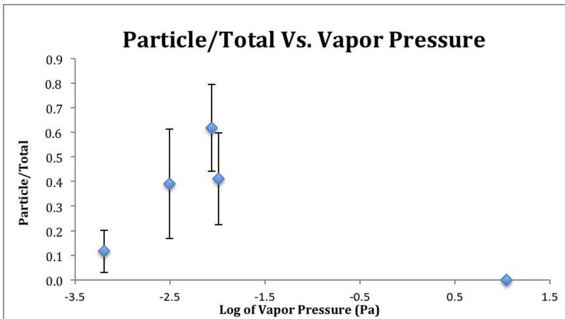
**Figure 4.2:** Illustrates the overall dependence of target nitrophenol partitioning with vapor pressure (Table 4.8). The average particle to total ratios of each nitrophenol compound from the ten parallel measurements shown in Table 4.5 are plotted against the log of vapor pressures. The error bars represent the standard deviations.
