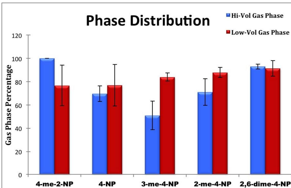
**Figure 4.5:** Comparison of the average percentage of the gas phase nitrophenols between the High-volume filter sampling and the denuder-filter methods (acquired by Facca). The average gas phase percentages are obtained from four sampling events where the two methods were sampled in parallel. Gas phase = (mass on XAD filter – mass on quartz filter)/ mass on XAD) x 100 %. The error bars represent the standard deviations
