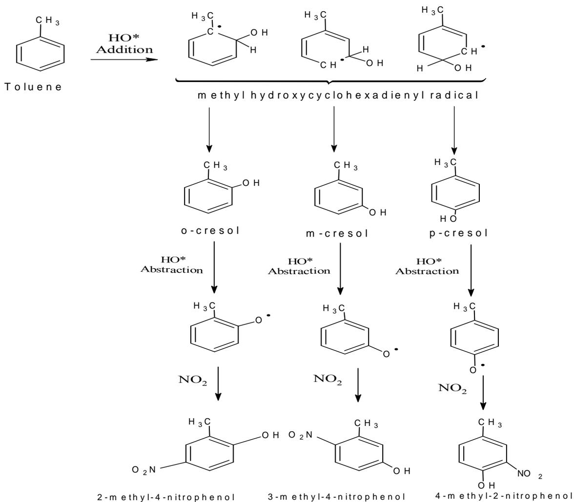
**Figure 2.3:** Reaction mechanism for formation of methyl nitrophenol from toluene (Forstner et al., 1997).
