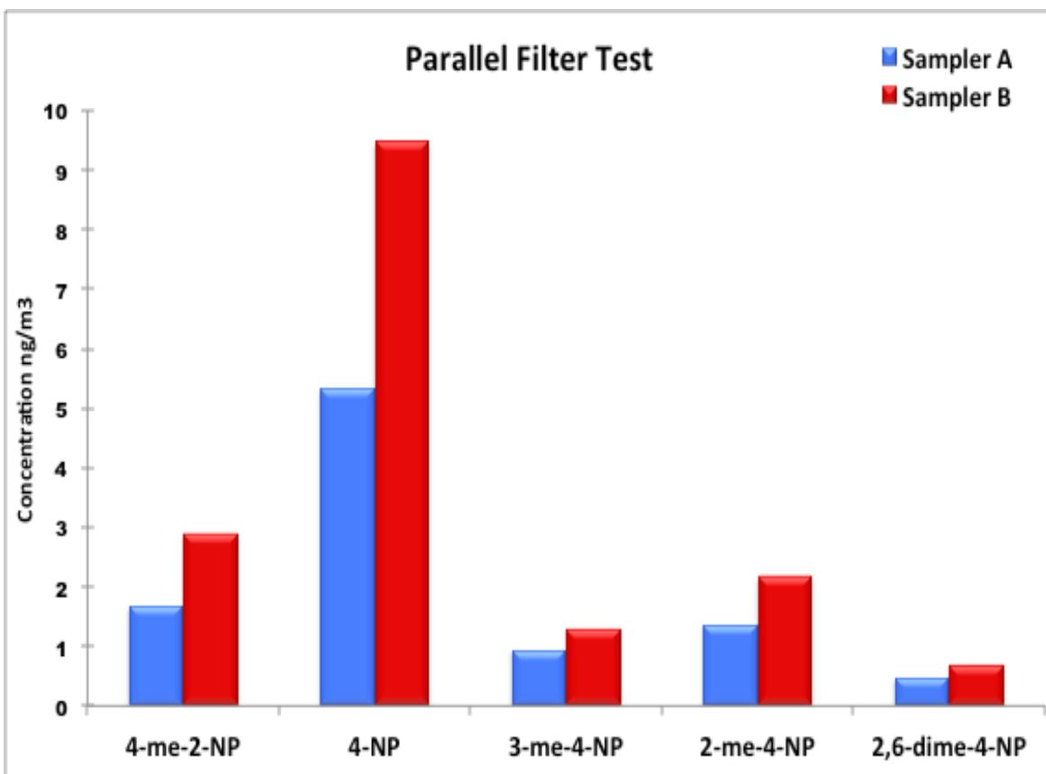
**Figure 4.1:** Comparison of target nitrophenol compounds' concentrations on two XAD coated filters sampled in parallel using two separate high-volume sampling units.
