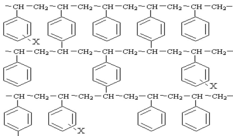
**Figure 2.1:** Polystyrene-divinylbenzene copolymer resin.
