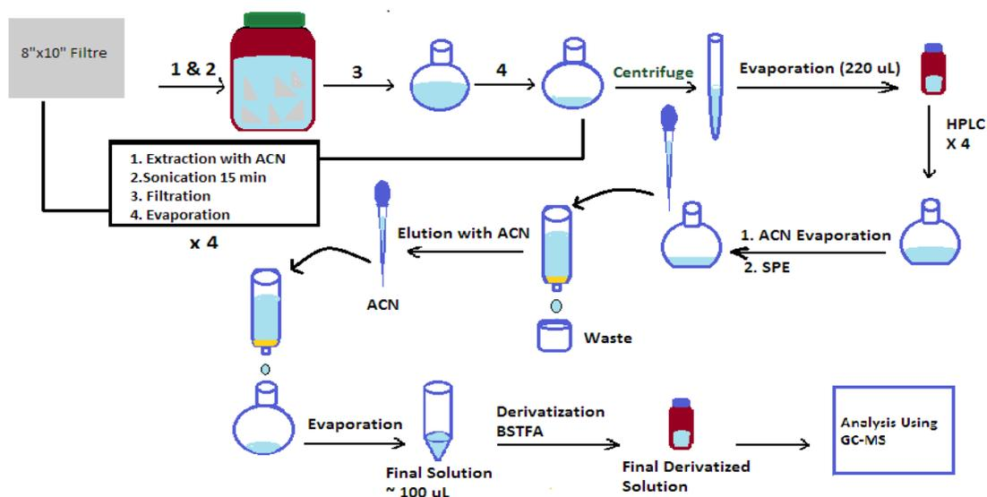
**Figure 3.1:** Schematic of the extraction procedure carried out for filter analysis.
