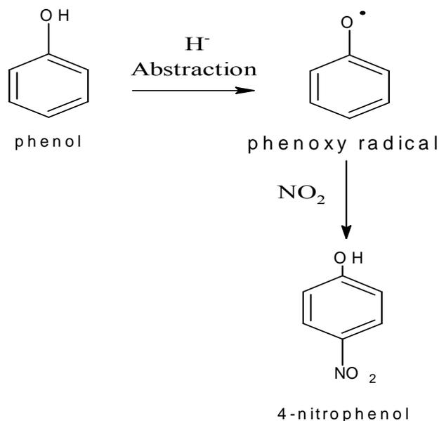
**Figure 2.5:** Formation mechanism of 4-nitrophenol from phenol (Atkinson et al., 1992).
